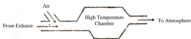
Thermal Exhaust Reactor
