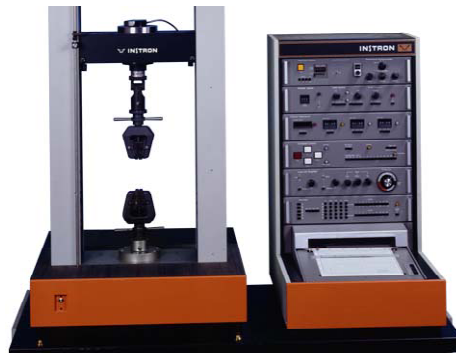
Instron model 1122 testing equipment with punch probe
