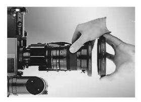
A type of filter that's much cheaper than glass is the gel. A gel is a small square or rectangular sheet of optic plastic used in front of the lens in conjunction with the matte box. (See below.) Professionals refer to these two basic filter types as round filters and rectangular filters.
