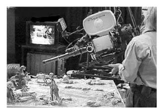
In the photo on the right, the camera operator uses a lens probe to film a miniature prehistoric setting that will later come to life in a full-scale effect. Although this is a film camera, it has a video viewfinder to provide immediate feedback on the image captured on film. (Note the video monitor).
