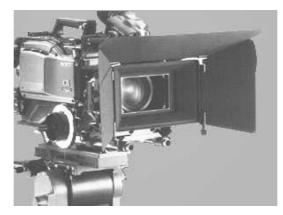
As we noted earlier, instead of using circular glass filters, you can insert into the matte box a comparatively inexpensive square or rectangular colored gel (gelatin filter) just in front of the lens. Note the photo on the left.
