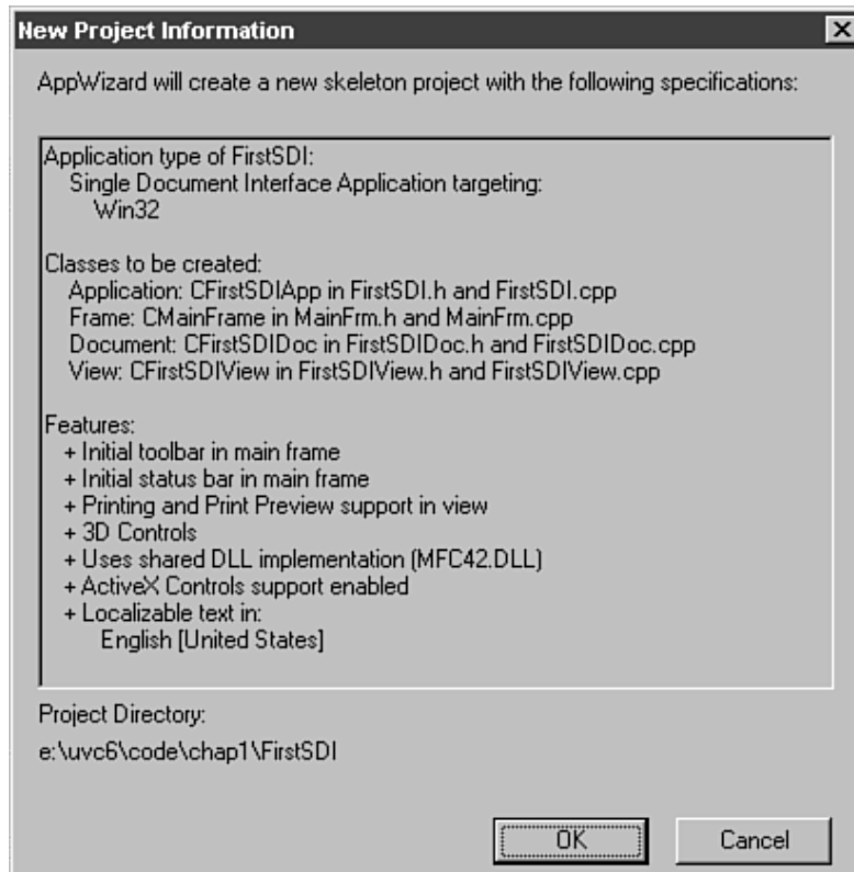
FIG. 1.11 When AppWizard is ready to build your application, you get one more chance to confirm everything.
