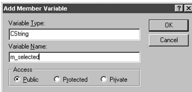
FIG. 2.14 Add a CString to your class to hold the string that was selected in the list box.
