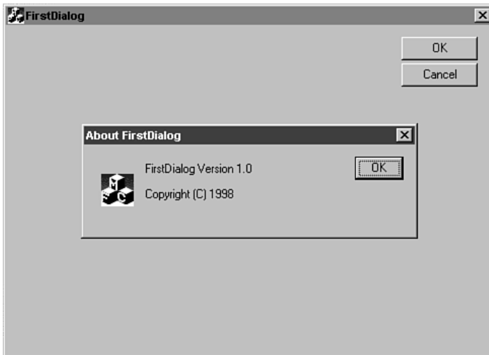
FIG. 1.21 The same About box is generated for SDI, MDI, and dialog-based applications
