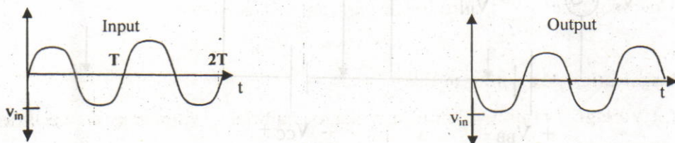
Fig 7.3 180^\circ phase shift between input and output waveform
