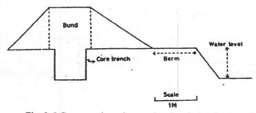
Fig. 2-5 Cross section of an earthen bund showing berm
