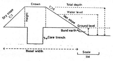
Fig. 2-4. Cross section of an earthen bund
