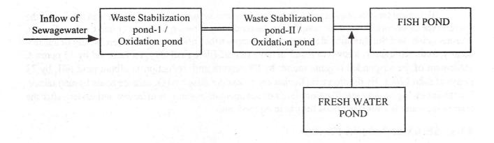
Fig. 4.1 Flow chart showing treatment of Seavage water for use in fish culture ponds.
