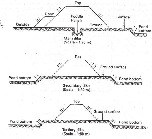
Fig. 2.3. Cross sections of some typical types of dikes.
