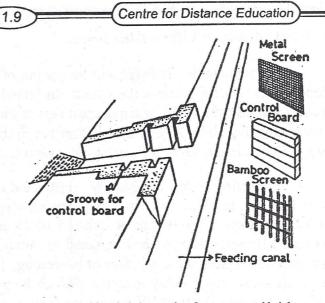
Fig. 2-6. Simple inlet made of concrete and bricks
