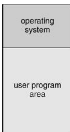
Figure 1.2 Memory layout for a simple batch system.
