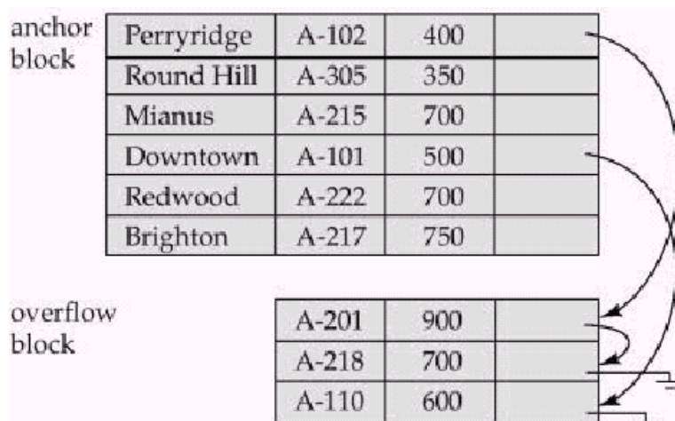
Figure: 9 Anchor-block and overflow-block structures
