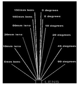
A telephoto lens (or a zoom lens operating at maximum focal length) has a narrow angle of view. Although no exact definition for a "telephoto" lens exists, we would consider the angles at the top of the drawing from about 5 to 10 degrees in the telephoto range. The bottom of the drawing (from about 45 to 90 degrees) represents the wide-angle range for this lens.
